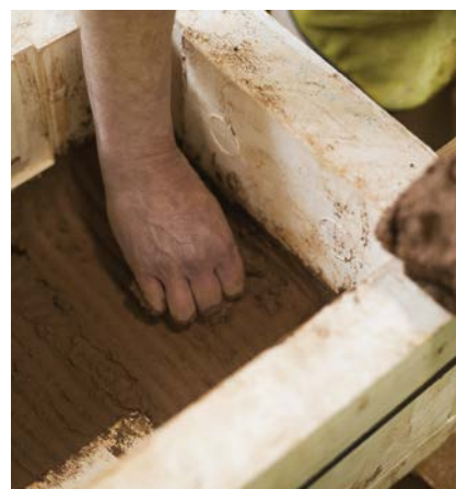
② Clay being applied to plaster mould. This process, called slip-casting, is designed to shape the clay into the required form before firing
